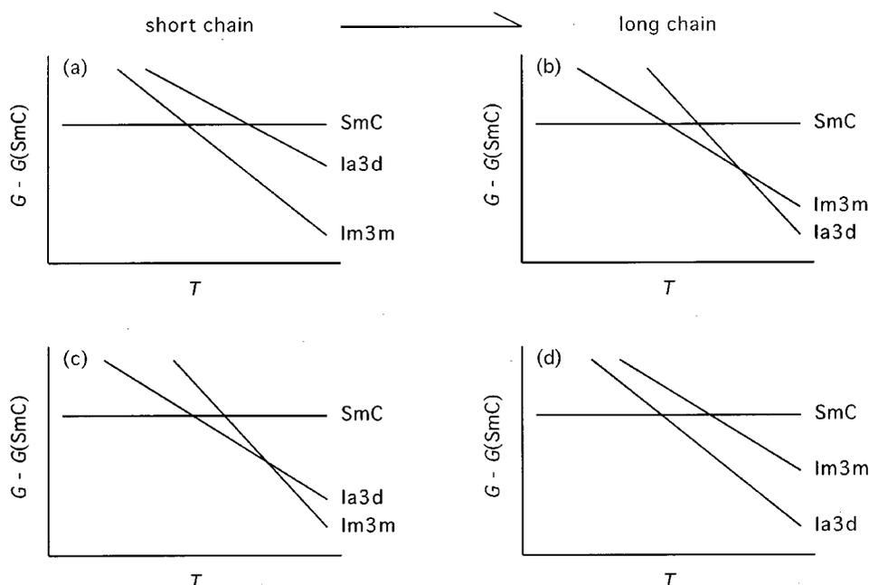
FIG. 8. Gibbs energy ( $G$ )-temperature ( $T$ ) diagrams showing possible phase sequences including two cubic ( $Ia3d$  and  $Im3m$ ) phases.
