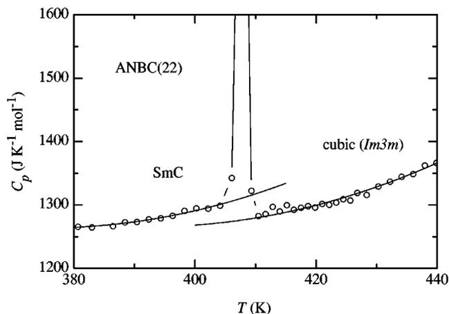
FIG. 4. Measured heat capacities of ANBC(22) around the Sm-C → cubic (*Im3m*) transition. Solid curves are smooth extrapolations of the heat capacities of the Sm-C and cubic phases.
