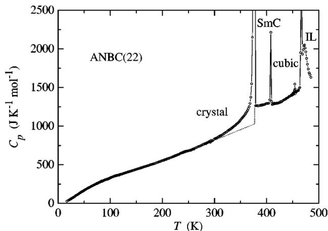
FIG. 2. Measured heat capacities of ANBC(22) in the whole temperature range. The isotropic liquid is denoted by IL. The assumed normal heat capacity (baseline) is drawn by a dotted curve.
