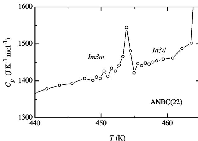
FIG. 5. Measured heat capacities of ANBC(22) around cubic (*Im3m*) → cubic (*Ia3d*) transition.
