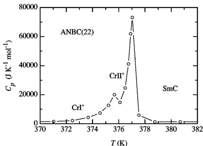
FIG. 3. Measured heat capacities of ANBC(22) in the melting region. Two crystalline phases are denoted by CrI' and CrII'.
